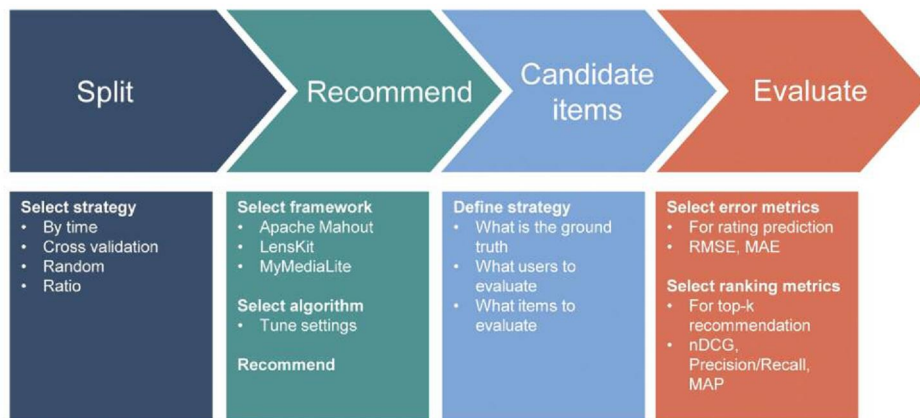
Figure 1: The RiVal evaluation pipeline. The toolkit's modular design means each module can be executed individually (i.e., only the evaluation module or only the data splitting module) or alternatively, the complete pipeline can be executed within RiVal.
