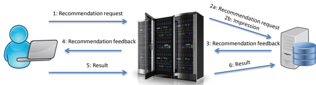
Figure 1: The flow of messages sent between a user reading an article, the Plista server, and the participant’s recommendation algorithm.
