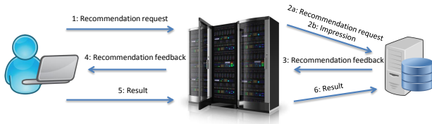
Figure 1: The flow of messages sent between a user reading an article, the Plista server, and the participant’s recommendation algorithm.
